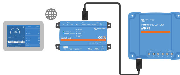
VictronConnect App connection via LAN or the internet (VRM portal) using a GX device (for example a Cerbo GX)
