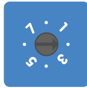
Rotary switch set to position 2
