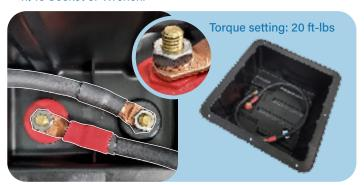
5) If installing Lithium battery, attach battery cables to posts on battery with appropriate hardware.
