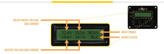
When the controller is powered up, the top line of the LCD display gives the voltage and the amperage coming in from the solar array, as well as the total power in watts. The bottom line of the display shows the battery voltage, and the amount of amperage the controller is sending to the battery bank, followed by what mode the charge controller is in.
