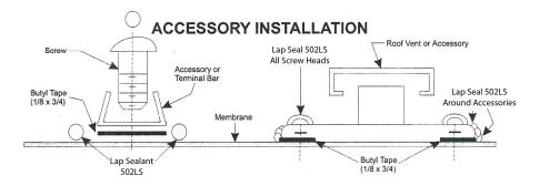
11. Caulk all screw heads, front and rear termination bar and all accessories. **NOTE: Only Butyl Tape can be used with this membrane to assure proper seal.**
