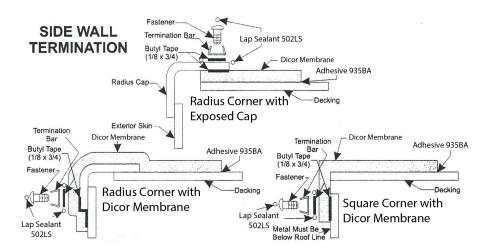
Apply butyl tape (BT-1834) to the termination molding. On the front of the vehicle, the front cap should lay on top of the membrane. Using a screw-type fastener, install the termination moldings –making sure there is sufficient roof structure. On the rear of the vehicle, the membrane should lay on top of the rear cap.
