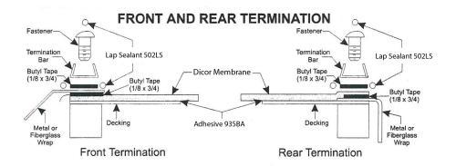
NOTE: Butyl tape should also be used under the membrane where it comes in contact with the unit body at the front, rear, and side terminations. See all termination drawings for correct butyl placement.
