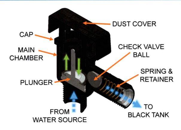
When the 571 Vacuum Breaker is functioning properly, the internal plunger will have free vertical travel within the main chamber. Contaminants or obstructions in the main chamber are the most common issue experienced with the 571 Vacuum Breaker.
