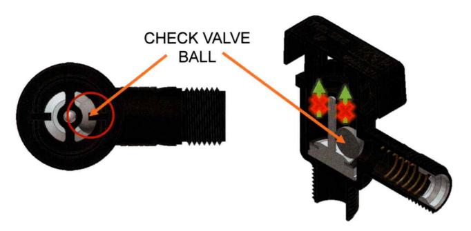
If pressure is present for an extended period, the check valve ball can migrate into the main chamber of the vacuum breaker. When this happens, vertical movement of the plunger is blocked, preventing a closed seal at the top, which allows water to flow around the plunger, over the cap, and onto the RV floor.
