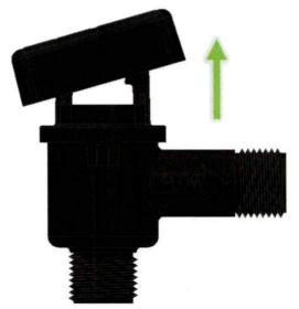
The first step is to remove the 571 Vacuum Breaker from their unit for inspection. According to RVIA code, it should be located somewhere easily accessible, above the highest flood plane of the RV (toilet rim). It is commonly found beneath the bathroom sink, but some manufacturers may choose to put it in a different location. In which case, you may need to contact your RV manufacturer.
