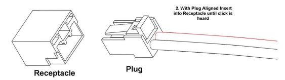
This is a detailed view of the Plug and Receptacle for plugging the Inside Plate Assembly into the Receptacle on the Bauer NE Housing.
