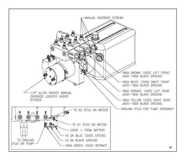
Note: All wire gauge sizes and breaker ratings noted are the recommended size. Larger gauge wiring and higher breaker rating may be used. There may be variances on specific systems supplied to OEM customers due to the exact makeup of the system.
