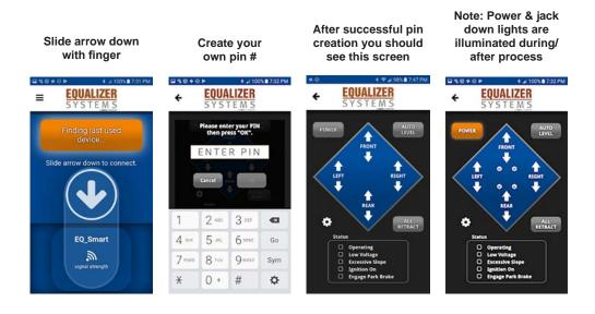
Note: The All Retract button will only retract the rear (and center jacks on a 6 point) on a trailer system.
