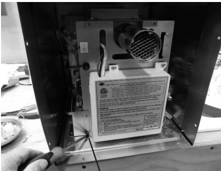
Remove two valve bracket screws and the one case screw
