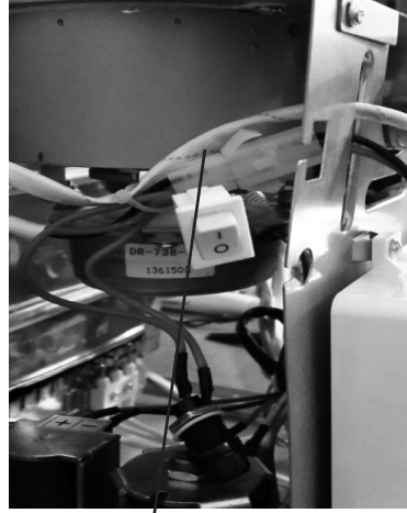
Disconnect red and black wire connector
