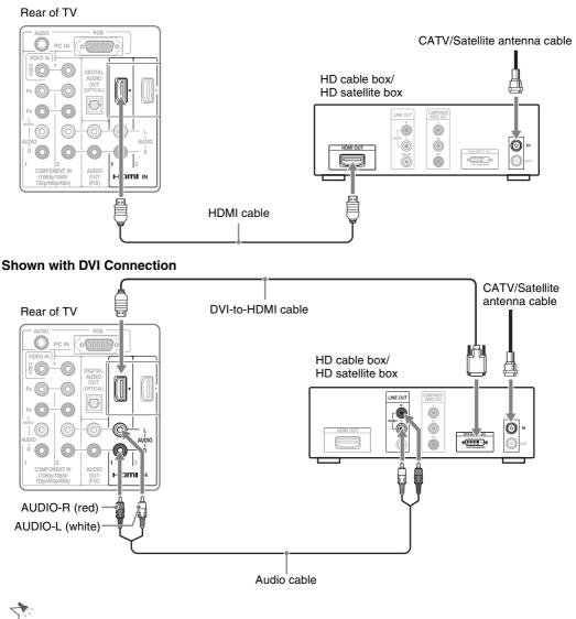
• If your equipment has a DVI output and not an HDMI output, connect the DVI output to the HDMI IN 1 (with DVI-to-HDMI cable or adapter) and connect the audio output to the AUDIO IN (L/R) of HDMI IN 1. For details, see page 7.
