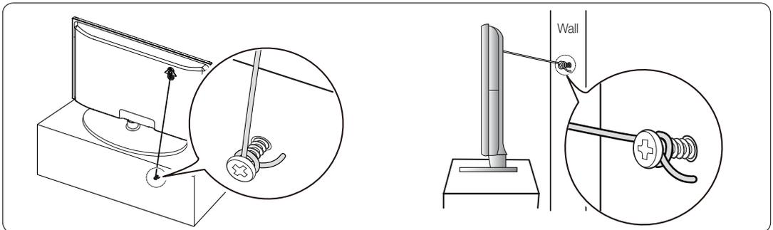
4. Verify all connections are properly secured. Periodically check the connections for any sign of fatigue or failure. If you have any doubt about the security of your connections, contact a professional installer.
