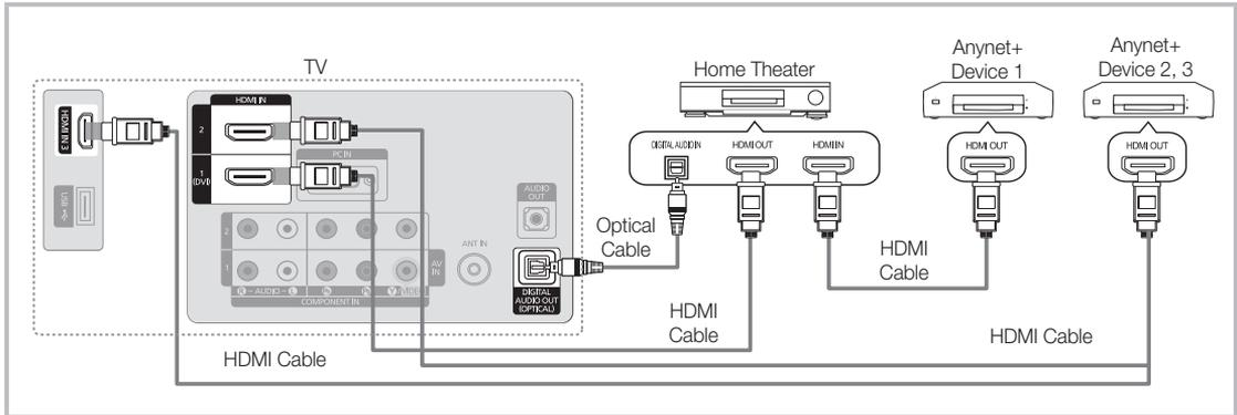
1. Connect the **HDMI IN (1 (DVI), 2 or 3)** jack on the TV and the **HDMI OUT** jack of the corresponding Anynet+ device using an HDMI cable.
