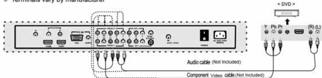
1. Connect LCD TV's YPbPr1 or YPbPr2 terminal to DVD's Video Out terminal .
