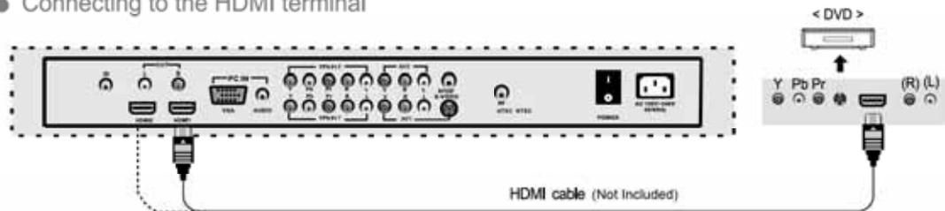
· Connecting from HDMI terminal to HDMI terminal.
