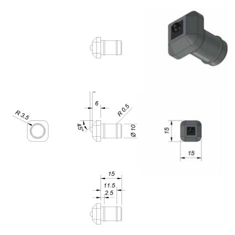
The extension eye is for mounting in a 10 mm hole. The eye has a 2000 mm cable with a mini Jack plug, which is to be plugged into the DP1V.
