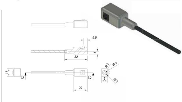
The extension eye is for surface mounting (with self adhesive tape on the back of the extension eye). The eye has a 2000 mm cable with a mini Jack plug, which is to be plugged into the DP1V.
