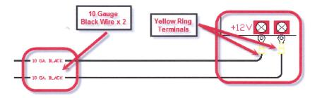
The power connection will be made via two 10 gauge wires, connected to the load side of the single 50A mini breaker, which the red 10 gauge slide out power is connected to. See below:
