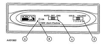
NOTE: If the gas does not ignite in 30 seconds, the gas safety valve of the refrigerator automatically closes and the GAS light flashes. To reset the controls, push the selector switch to the OFF position
