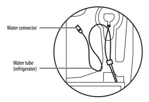
**3** Turn water on and check for any leakage.
