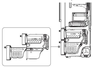
**2** Press the buttons in both slots at the same time, then pull out the freezer drawer until it stops again.
