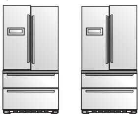
If the doors are uneven, first try leveling the freezer. See "Leveling your refrigerator" on page 10. If the doors are still uneven, raise the uneven door, then use a pair of pliers to insert the supplied fastener-ring in the gap between the hinge-grommet and the lower hinge. The number of fastener-rings needed depends on the gap.
