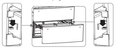
3 Lift the drawer off the rails and remove it.
