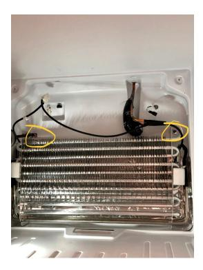
Remove two screws holding the cooling element to the back of the refer.
