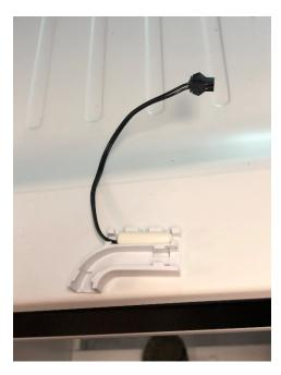
Unplug the quick connector from the back of the refer. Gently pull up on the thermostat to remove it from the housing.
