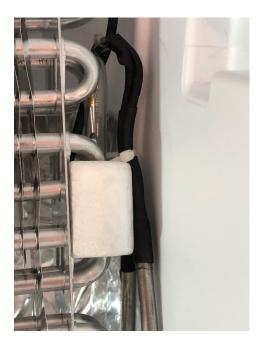
Cut two zip ties holding the wires on either side of the cooling unit and remove the styrofoam spacers. You will need to keep them for reuse.
