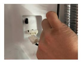
Disconnect defrost heater quick connector from the back of the refer.
