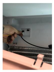
Disconnect quick connect on the back of the refer for the fan and remove back panel housing containing fan.
