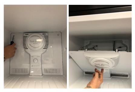
Remove two screws in top right and left corners of the back of the fridge. Pull forward and down to remove back cover. Be careful not to pull down to far because of connected components.
