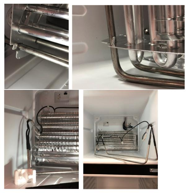
Bend up the tabs securing the defrost heater to the cooling element and pop the defrost heater off of the bottom of the cooling unit.
