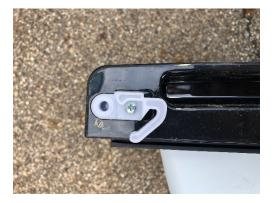
Once you have reinstalled the correct insert and you have reinstalled the middle hinge, set the freezer door on the hinge. Ensure that you do not let it fall off while the top hinge is not reinstalled.
