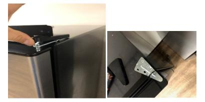
Next carefully remove the middle hinge bracket from the refer. Ensure that when you remove the two bolts from the middle hinge that you do not let the fridge door fall and get damaged. Ensure that you do not lose either of the plastic washers on the hinges as they help keep the door opening and closing smoothly and they ensure proper spacing of the door. Remove fridge door and set aside.
