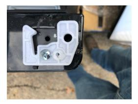
Once you have reinstalled the bottom hinge and moved the insert to the correct side, set the refer door back on carefully and close the door so it will stay in place.
