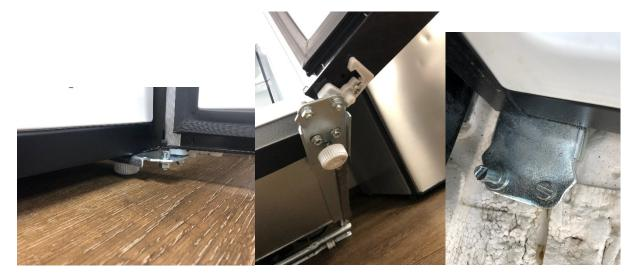
On the bottom of the refrigerator door there is a plastic soft close insert that must be taken off of the door, flipped over and moved to the other recessed pocket on the other side of the door. Uninstall by removing one screw and insert. Reinstall on the opposite side of the door in the recessed pocket for the insert and secure with the same screw you removed from the other side.
