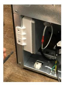
Remove 2 philips screws holding the Control Board box to the left hand side of the refer.
