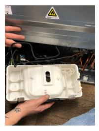
Gently pull pan out and remove evaporation heater lines from the pan. They are retained by plastic slide in tabs.
