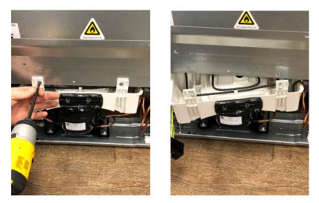
Remove 2 philips screws holding condensation catch pan.
