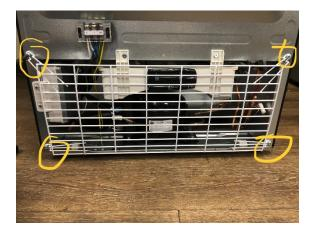
Remove 4 hex head Philips screws holding the protective back cover in place.
