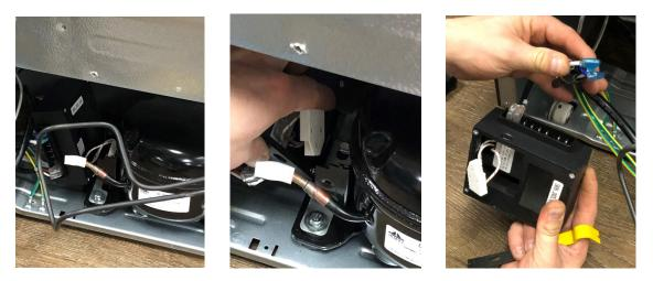
Once the board is loose, remove the socket plug attached to the side of the compressor. Do Not Pry on the connector, it will cause damage to the compressor. It will come off with light pressure. Once free, remove spade connectors.
