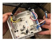
Remove the retaining Philips screw holding the circuit board in the box and the board will pop out. Once it is removed, remove the spade connectors and the ribbon cable connectors.
