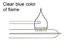
If the flame appearance is not correct (e.g. the flame is yellow or the shape is constantly changing and/or flickering or if the flame is touching metal surfaces inside the burner box – do not use the GAS mode and contact your dealer or authorized Atwood service center.
