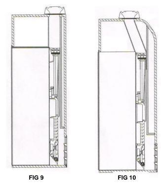
For installations where the depth of the enclosure is greater than 26 inches, additional baffling may be required to direct the airflow thru the absorber and condenser section of the refrigerator as shown in Fig 10.
