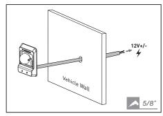
2. Fix the mounting bracket onto the marked location using two flat self-tapping screws provided.
