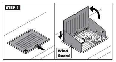
• Lift the Cover from the center slot. Raise it completely, then drop the Cover down to lock into the back of the Cooktop.
