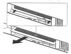
5 Push the tab to release the light cover and carefully pull it up from the front edge.
