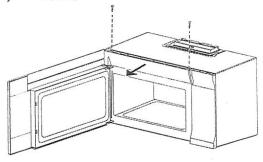
4 Remove the charcoal filter by pushing it inwards, then lift up and pull it out of the microwave.
