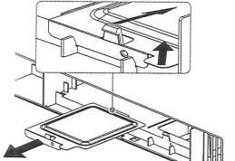
6 Remove the LED module and replace only with an equivalent 1.2 watt LED bulb.
