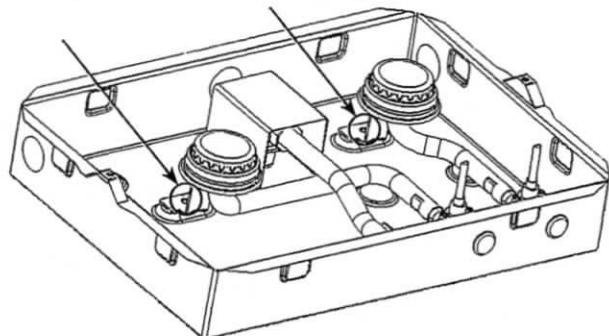
3. Check and clean burner/venturi tubes for insects and nests. Never use a wire brush or metallic item for cleaning burner ports or orifices.
