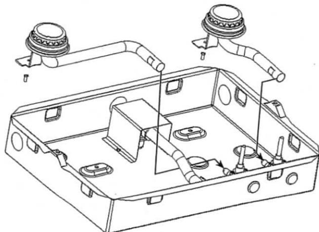
**Valve outlets must be securely seated within the burner tubes before finally re-installing the cooktop. Failure to reassemble the burner tubes correctly may result in a fire or an explosion, causing property damage, personal injury or death.**
