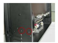
d. To take 2 pcs screws off of the motor supporting picture below.
