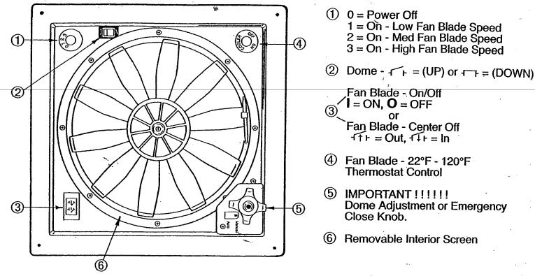
Notice: Do not leave fan in active automatic mode while rig is stored or unattended for long periods — high winds, other unusual conditions or obstructions may prevent closing: resulting leakage could cause damage.
