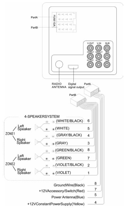
1. This player can only be used by the 12V DC cathode grounding electrical system.
