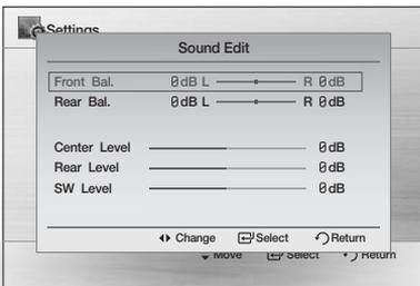
Press the ▲▼ buttons to select and adjust the desired speaker.
