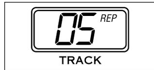
2. Press the repeat button two times while a track is playing. REP will be displayed. When the last track on the disc has finished playing, play will start over at track #1.
