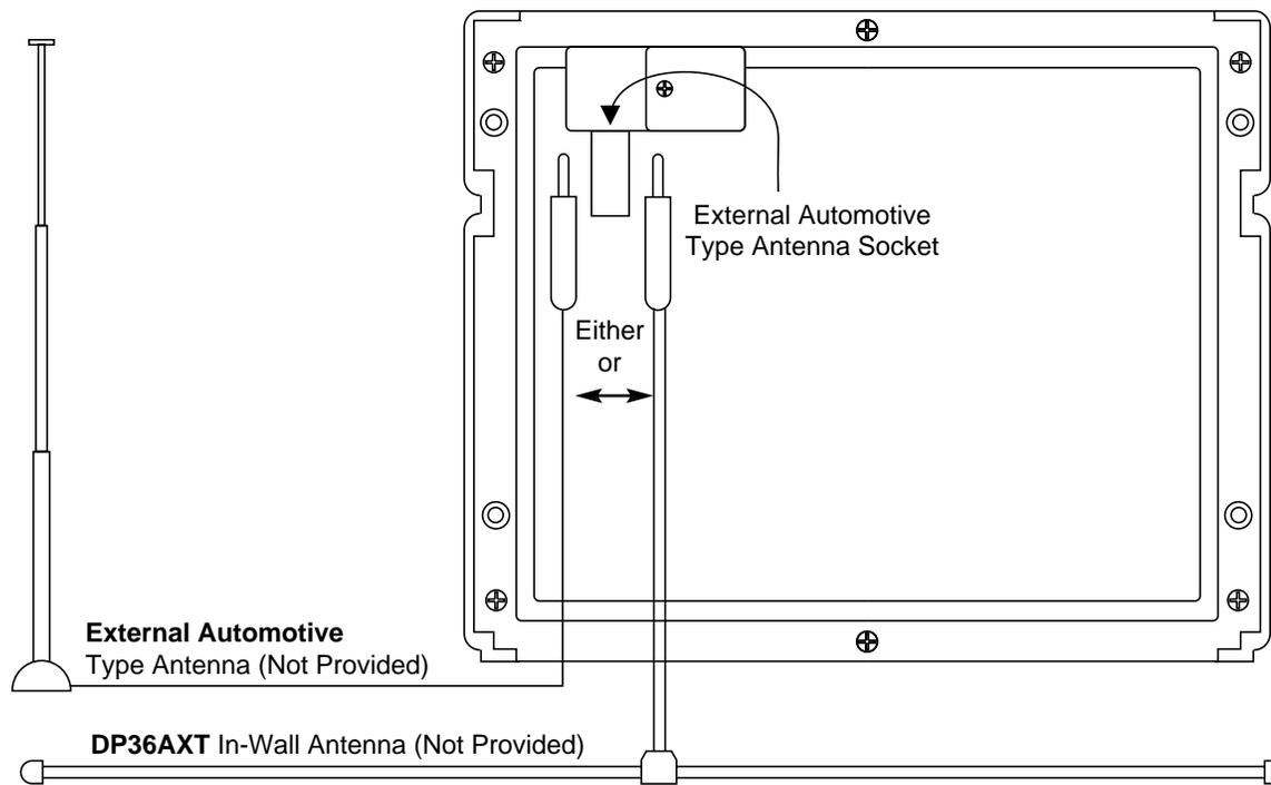
The LS7500CD have a provision for a standard automotive antenna. If an automotive antenna is used, plug the male plug from the antenna into the female receptacle provided on the unit.
