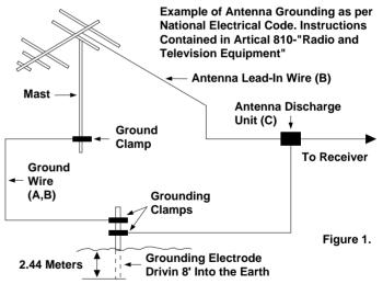
**A)** Use No. 10 AWG (5.3mm2) copper, No 8 AWG (8.4mm2) aluminum, No. 17 AWG (1.0mm2) copper clad steel or bronze wire, or larger, as ground wire.
