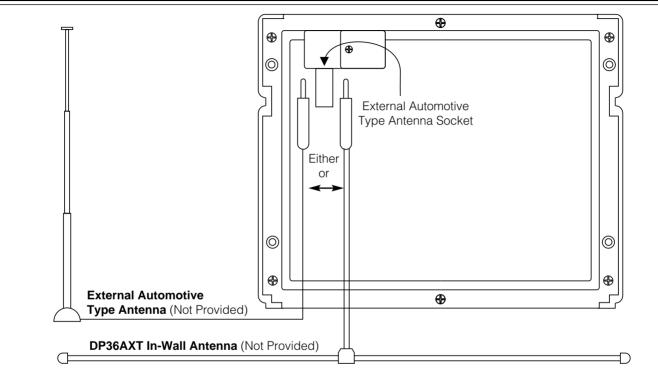
The LS6100 has a provision for a standard automotive antenna. If an automotive antenna is used, plug the male plug from the antenna into the female receptacle provided on the unit.
