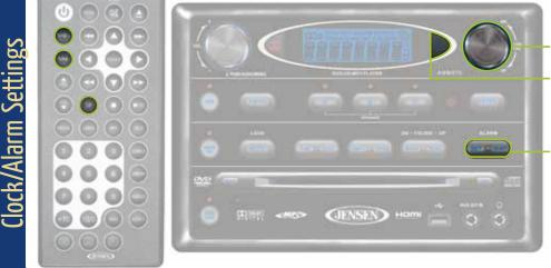
TUNE/TRACK: Rotate UP or DOWN to adjust HOUR and MINUTES once in CLOCK MODE or ALARM SETTING MODE.
