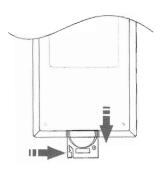
Insert the battery into the receptacle.
