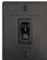
Power switch into wall plate
