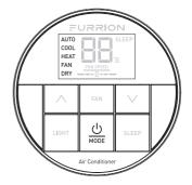
After the thermostat is turned on, press the (b) button repeatedly to toggle through the available modes. The activated mode icon and temperature set-point will be displayed on the LCD. The thermostat will transmit the last selected operation mode command to the control box after 2 seconds without any operation.
